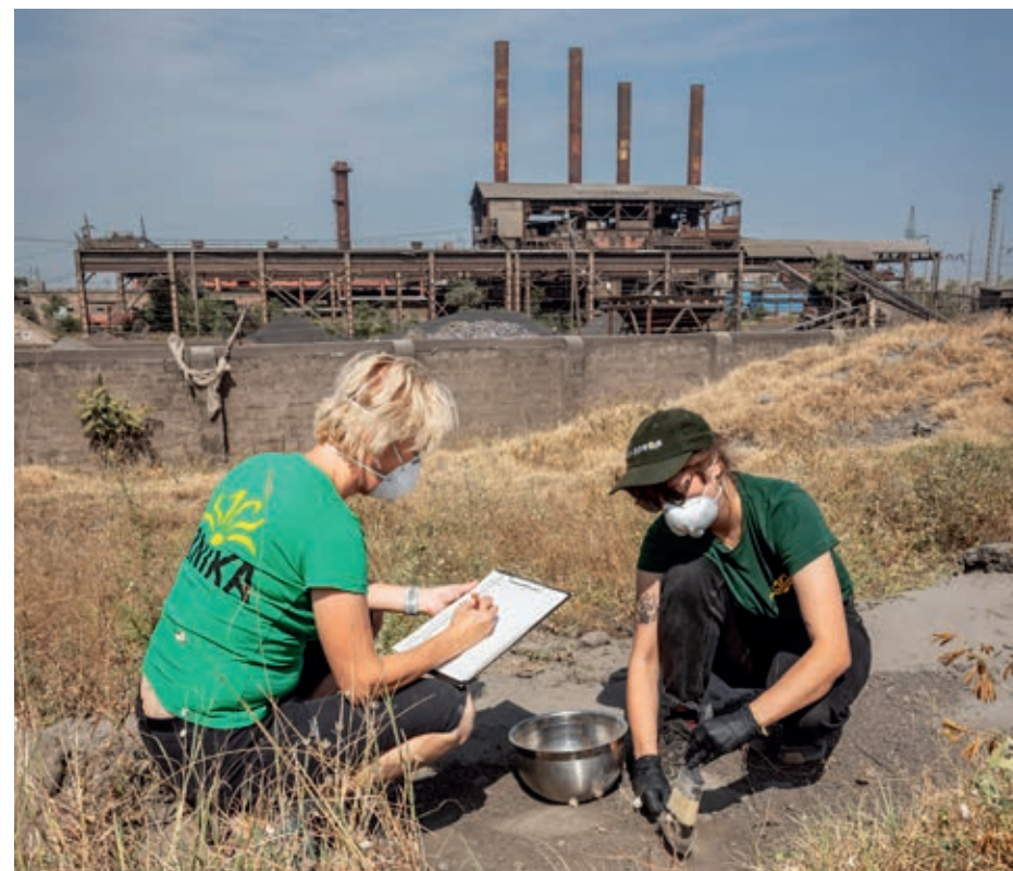
Photo 2.6: Dust sampling from the road between cement and ferro-alloys plants in Rustavi. Photo: Ondřej Petrlík
