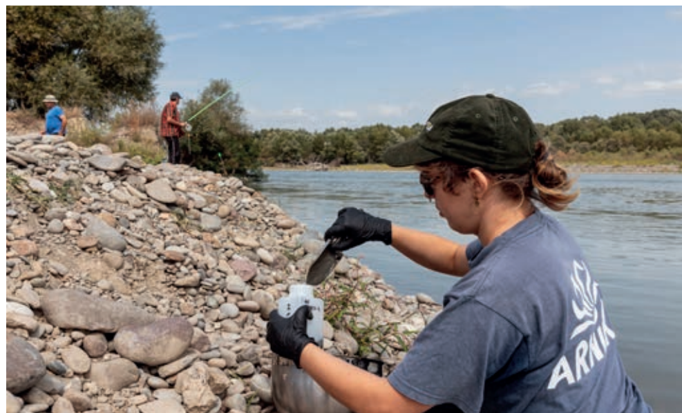
Sediment sampling in the Mtkvari River downstream from the wastewater treatment effluent discharge. Photo: Ondřej Petrlík
